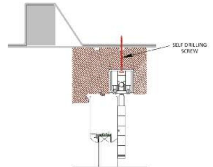
■ Your Bi-folding door must be supported from the top with adequate fixing points or your frame will sag in the middle. This in turn will impede the doors from opening or closing correctly and will affect the weatherseals and damage the doors and internal flooring.
